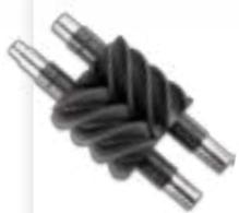
**1** The unique Z-seal design guarantees 100% oil-free air. The quality of the air is Class Zero certified by TÜV authorities. The compressor operates at safe running speeds and there is no contact between the rotors.
